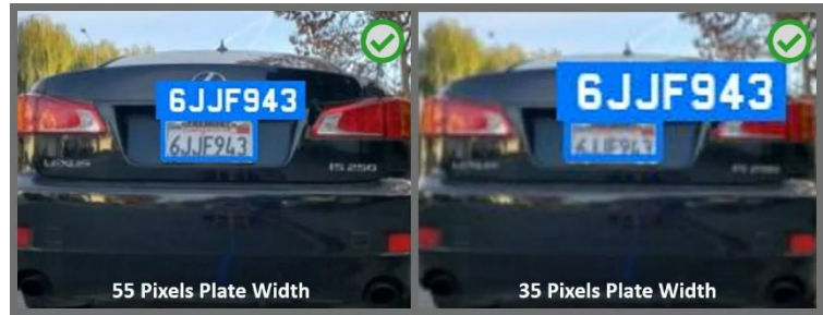
Figure 2-4 Plate clarity at differing pixel counts
